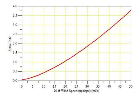
**Figure 9-6** – The Active Ratio calculated in BehavePlus is the ratio of the simulated to threshold crown fire rate of spread (ROS). Although BehavePlus does not directly calculate the Crowning Index (CI), it can be seen here as the 20-ft wind speed at which AR = 1, which is 19.1 mi/h. BehavePlus does not use slope steepness in its calculation of crown fire ROS, whereas NEXUS does, so the NEXUS-calculated CI is 18.6 mi/h.
