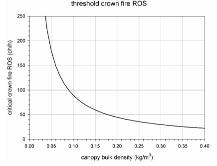
**Figure 9-4** – The critical (threshold) crown fire rate of spread is a function of canopy bulk density. Fully active crown fire is possible when the simulated crown *ROS* exceeds this threshold value. For our example fire modeling environment (*CBD* =  $0.15 \text{ kg/m}^3$ ), the threshold crown fire *ROS* = 59.7 ch/h (20 m/min).
