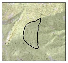
**Figure 5-1** – A slope is a terrain feature of uniform steepness and aspect. The area shown here is a slope that is east-facing and at a uniform steepness of 30 percent.
