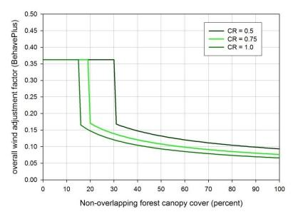
**Figure 6-4** – BehavePlus' overall wind adjustment factor as a function of canopy cover for three values of crown ratio (CR). Stand height is 30 m. The discontinuity in WAF occurs where crown filling fraction falls below 5 percent.
