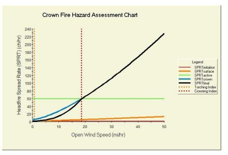
**Figure 9-8** – Crown fire hazard assessment chart in NEXUS for the example fire modeling environment, showing the TI and CI as dotted vertical lines and the final (overall) rate of spread as a black line.
