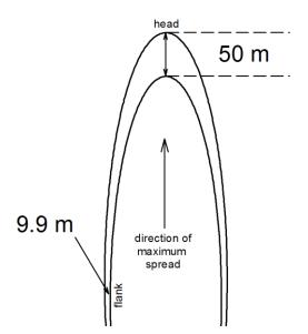
**Figure 1-11 –** The spread rate of the flaming front is its linear rate of advance in the direction perpendicular to the flaming front. The curving lines represent the position of the flaming front at two points in time that are just one minute apart. Spread rate is greatest at the head of the fire and decreases around the perimeter.
