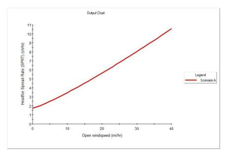
**Figure 7-11** – Graphical NEXUS output showing simulated surface fire rate of spread over a range of 20-ft wind speed.
