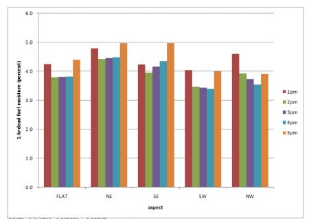
**Figure 4-8** – Effect of time of day on 1-hr timelag class moisture content. Different aspects experience their lowest 1-hr *MC* at different times of day, and moisture content can change quickly in just one hour.
