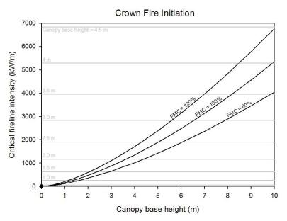
**Figure 4-13** – Critical (threshold) fireline intensity required to initiate crown fire as a function of canopy base height and foliar moisture content (*FMC*).
