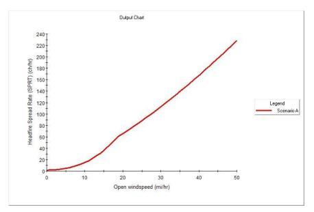
**Figure 9-15** – Output chart for final rate of spread (ch/h) over a range of wind speeds from 0 to 50 mi/h. To see these results in tabular form, simply switch to the *Output Table* tab; all settings from the chart are also applied to the table.
