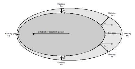
**Figure 1-8** – Sections of this simple fire perimeter can be classified by the orientation of the flaming front (dark arrows) with respect to the direction of maximum spread (gray arrows). The black dot represents the origin of the fire and is located at the rear focus of the ellipse.
