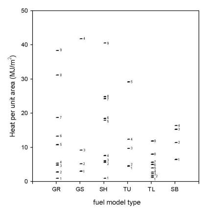
**Figure 1-12** – Surface fuel *HPA* values for the 40 fire behavior fuel models (Scott and Burgan 2005). Fuel models for each fuel model type are listed in a single column. This chart assumes 6% 1-hr, 7% 10-hr, and 8% 100-hr timelag moisture content values; live herbaceous moisture content is 60%; and live woody moisture content is 90%.
