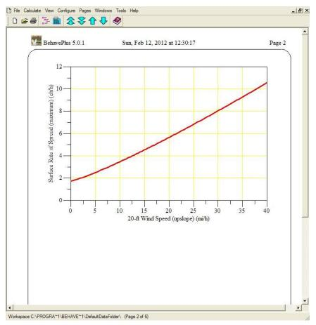
Figure 7-9 – Surface fire rate of spread over a range of 20-ft wind speeds.
