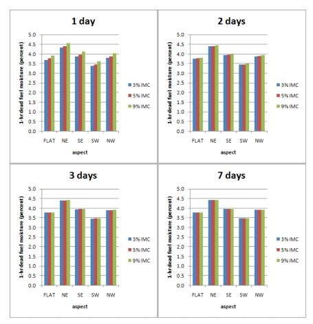
**Figure 4-7–** Effects of initial MC and length of conditioning period on 1-hr timelag class moisture content. Final 1-hr MC stabilizes after just 1-3 days, regardless of initial MC. Inputs: 50 percent canopy cover, 40 percent slope, 2 pm, hot, dry conditions.
