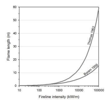
**Figure 1-17 –** Two mathematical relationships are commonly used to estimate flame length from fireline intensity; the models provide very different estimates of flame length for *FLI* values greater than 1000 kW/m. Thomas' (1963) model is most commonly used for estimating crown fire flame length, whereas Byram's (1959) model is used for surface fires.
