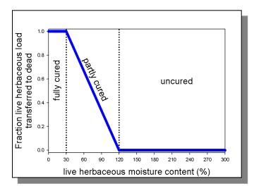
**Figure 4-12**—Operational fire modeling systems use this simple straight-line relationship between live herbaceous moisture content and the fraction of load transferred to the dead category.
