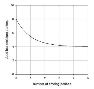
**Figure 1-19** –During one timelag period, dead fuel moisture moves 63% of the way from the original fuel moisture to the new equilibrium moisture content.
