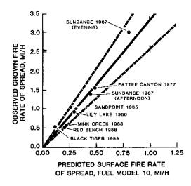
**Figure 8-1** – Wildfire data points used in Rothermel's (1991) correlation between observed crown fire spread rate and predicted surface fire spread rate (using certain inputs).
