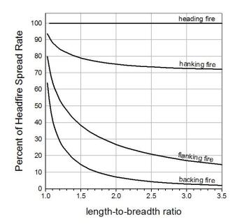
**Figure 1-21 –** Using the simple ellipse model of fire shape, spread rate around the perimeter of a fire can be related to the head fire spread rate. To use the chart, trace a vertical line from the X-axis, at the appropriate length-to-breadth ratio, to the desired spread direction—head, hank, flank, or rear (back). At the appropriate line, read the fraction of headfire spread rate from the Y-axis.
