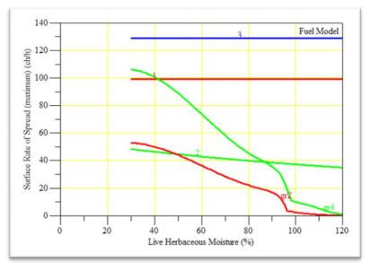
**Figure 4-11** – Surface fire rate of spread as a function of live herbaceous moisture content (*LHMC*). Fuel models 1 and 3 do not have a live herbaceous component and therefore are unaffected by *LHMC*. Fuel model 2 is a static model, so the effect of *LHMC* is small. Fuel models GR2 and GR4 are dynamic, so rate of spread is strongly affected by *LHMC*.
