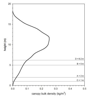
**Figure 3-1** – Canopy base height as estimated using several methods for a destructively sampled canopy fuel profile for a Douglas-fir / lodgepole pine stand on the Salmon-Challis National Forest. The 25<sup>th</sup> percentile crown base height (A) is 2 m. The mean crown base height (B) is 5 m. The height above ground where canopy bulk density exceeds 0.01 kg/m<sup>3</sup> (C) is 1 m. The CFSCC Version 1.0 estimates *CBH* for this stand as 6.2 m.
