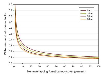
**Figure 6-3** – With-cover wind adjustment factor as a function of canopy cover (percent) for three different stand heights. This chart is for a crown ratio of 1.0, which is assumed in FARSITE and its related geospatial fire modeling systems.
