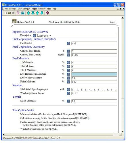
**Figure 9-12 –** The BehavePlus worksheet resulting from the settings described in figures 9-9 through 9-11. Use the guide button (arrow) to enter 20-ft wind speed values from 0 through 50 mi/h in steps of 1 mi/h.
