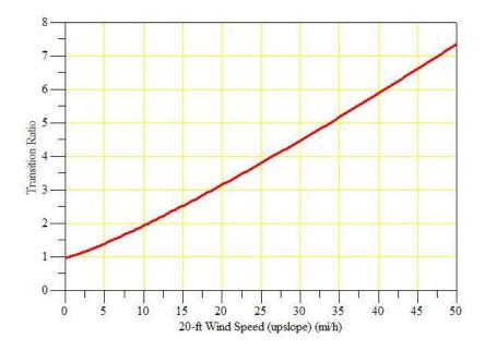
**Figure 9-3** – The Transition Ratio calculated in BehavePlus is the ratio of the simulated to threshold fireline intensity. Although BehavePlus does not directly calculate the Torching Index, it can be seen here as the 20-ft wind speed at which TR = 1, which is again between 0 and 1 mi/h.
