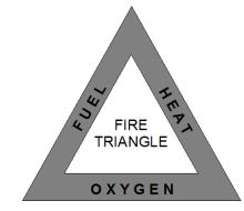
**Figure 1-3 –** The Fire Triangle. Fuel, heat, and oxygen are the required elements for fire. Remove any one of those elements and fire cannot continue.
