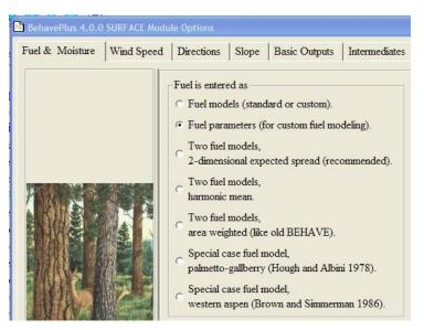
**Figure 22-2** – The SURFACE module options dialog box is used to specify how fuel is entered. To create a custom fuel model in BehavePlus, first set the "Fuel is entered as" button to "Fuel parameters (for custom fuel modeling)".
