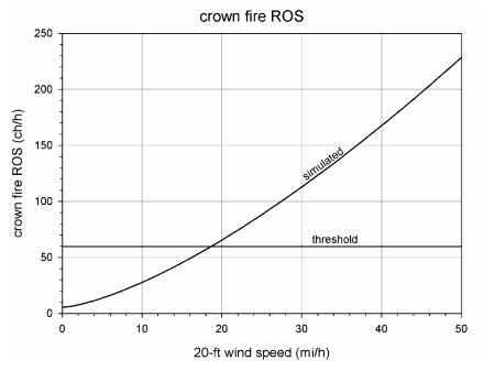
**Figure 9-5** – The Crowning Index is the 20-ft wind speed at which the simulated crown fire rate of spread (*ROS*) equals the threshold crown fire *ROS*. In this example, that occurs at a wind speed of 18.6 mi/h (for crown fire *ROS* as simulated in NEXUS).
