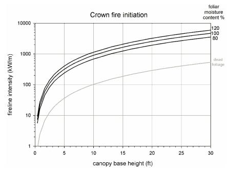
**Figure 9-1** – Van Wagner's (1977) crown fire initiation model determines the threshold fireline intensity required to initiate crown fire from canopy base height and foliar moisture content (*FMC*). Typical values of *FMC* range from 80-120 percent and have little effect on critical fireline intensity. Dead foliage still attached to branches has much lower moisture content (here assumed to be 10%) and therefore is more prone to ignition.
