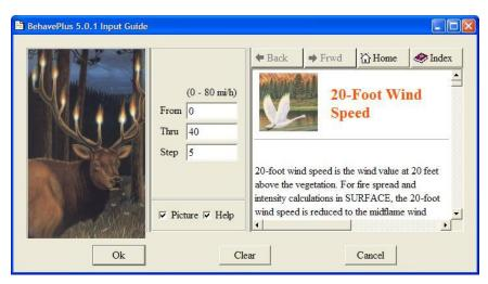
**Figure 7-8** – Input guide for setting 20-ft wind speed to range from 0 to 40 mi/h by steps of 5 mi/h.
