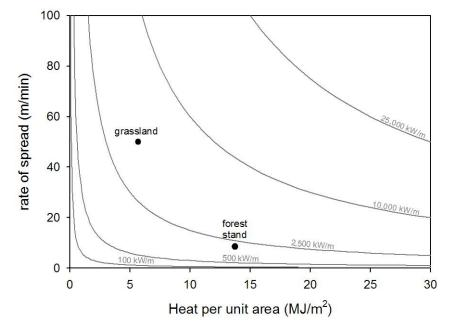
**Figure 1-14** – A fire behavior characteristics chart can depict three quantitative fire behavior characteristics at once. The Y-axis represents flaming front spread rate, the X-axis represents heat per unit area, and the curving lines represent fireline intensity.
