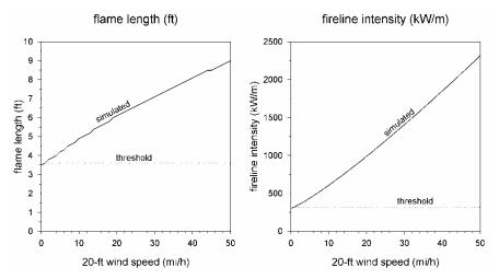
**Figure 9-2** – The Torching Index is the 20-ft wind speed at which the simulated fireline intensity (or flame length) equals the threshold value. In this example (see Table 9-1), this transition occurs when the wind speed is between 0 and 1 mi/h. In other words, crown fire initiation can occur with little or no wind.
