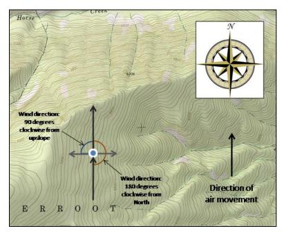
**Figure 6-5** – Illustration of cardinal wind direction (with respect to north) and relative wind direction (with respect to slope).
